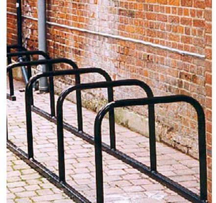
The VELOPA Sheffield Cycle Toastrack is a floor fixed cycle rack based upon the Sheffield Cycle Stand. The Sheffield Cycle Toastrack consists of Sheffield Cycle Stands welded at 800mm centres to floor fixed box section rails. The benefits of a Cycle Toastrack over individual stands are reduced installation costs and pre-determined gaps between stands, each stand is suitable for parking two bicycles. The Sheffield Toastrack is ideal where cycle parking in large numbers is required.
