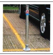
Designed for use delineating the edge of car parking spaces, the Sprung Boundary Post has a spring incorporated into the base which allows it to absorb low speed impacts and return to it's original upright position.
