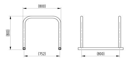
The VELOPA Sheffield Cycle Toastrack is a floor fixed cycle rack based upon the Sheffield Cycle Stand. The Sheffield Cycle Toastrack consists of Sheffield Cycle Stands welded at 800mm centres to floor fixed box section rails. The benefits of a Cycle Toastrack over individual stands are reduced installation costs and pre-determined gaps between stands, each stand is suitable for parking two bicycles. The Sheffield Toastrack is ideal where cycle parking in large numbers is required.
